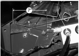
Adjust the feeder house faceplate so that the draw-bolts measure 7" (178 mm) as shown.
