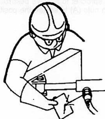
CHECK PROPERLY FOR LEAKS
