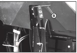
Figure 2: Wing Lock Spring Handle in Locked Position
