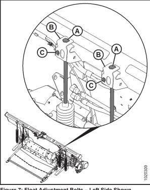
Figure 7: Float Adjustment Bolts – Left Side Shown
