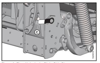
Figure 3: Float Unlocked - Right Side Shown
