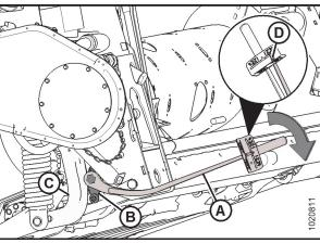
Figure 6: Checking Float - Left Side Shown
