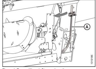
Figure 4: Torque Wrench Storage Location
