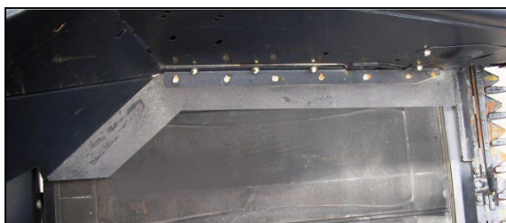
DEFLECTOR AFTER TRIMMING
