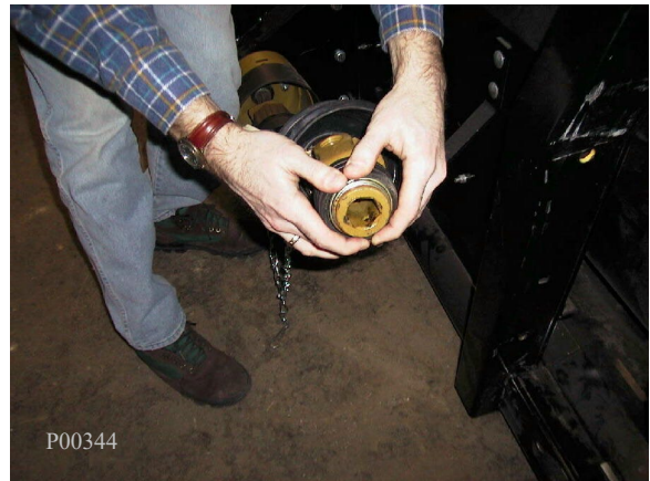
Drive Shaft to Header Installation
