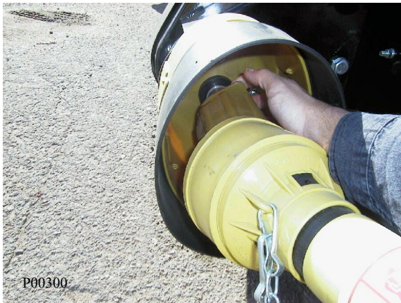
Drive Shaft to Header Installation
