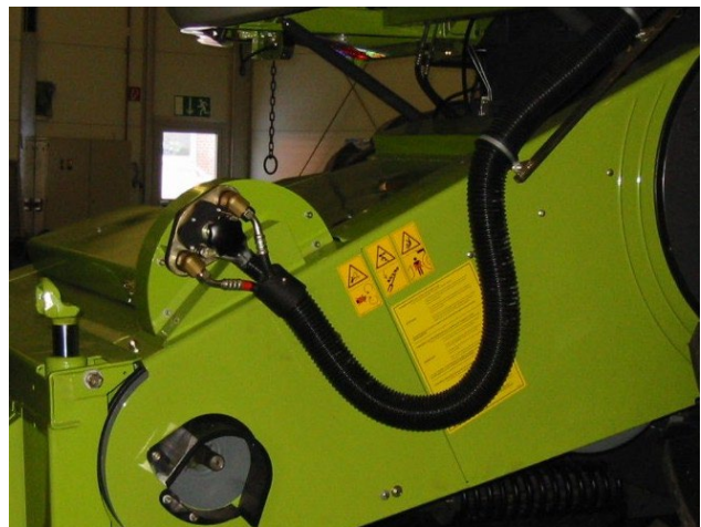
Feeder house Multi Coupler in Storage
