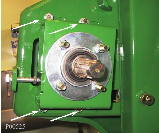
Drive Shaft Bracket Bolts
