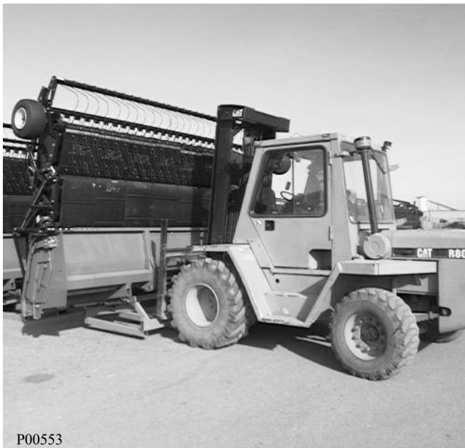
Lifting Header/Pickup In Shipping Position
