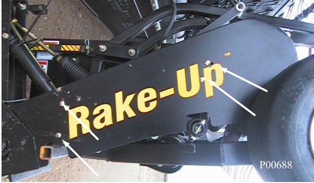
Rake-Up Drive Shield Removal
