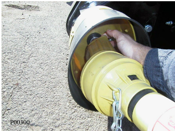
Drive Shaft to Header Installation
