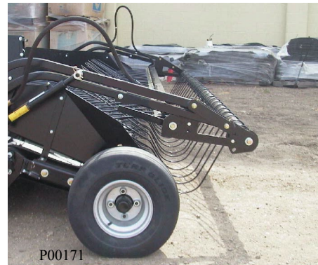
Hold-down Adjusted for Short Crops
