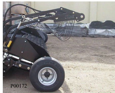
Hold-down Adjusted for Average Crops
