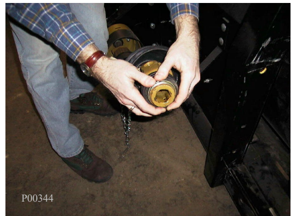
Drive Shaft to Header Installation
