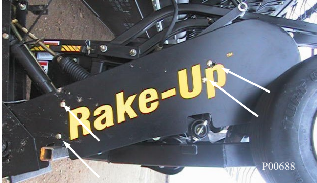
Rake-Up Drive Shield Removal
