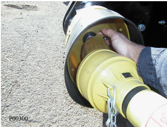
Drive Shaft to Header Installation
