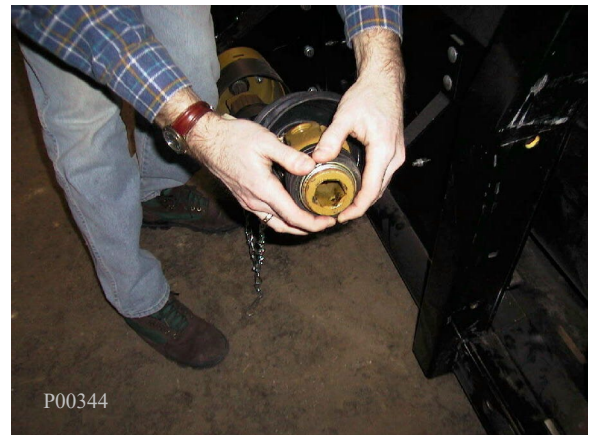
Drive Shaft to Header Installation
