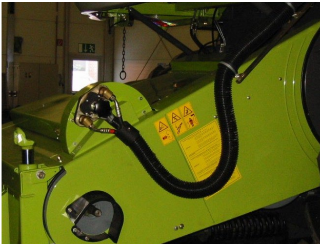
Feeder house Multi Coupler in Storage
