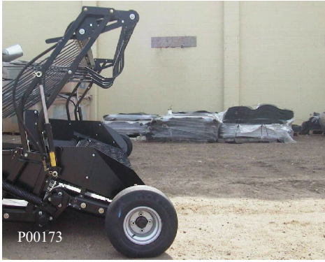
Hold-down Adjusted for Heavy Crops
