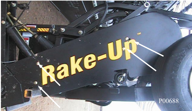
Rake-Up Drive Shield Removal
