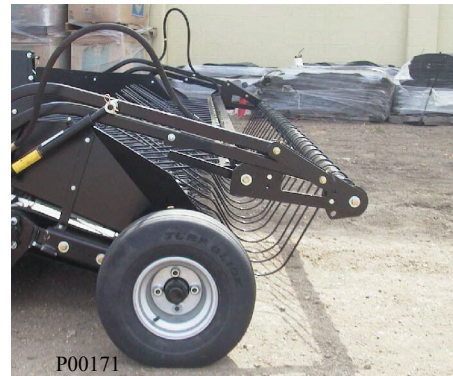
Hold-down Adjusted for Short Crops
