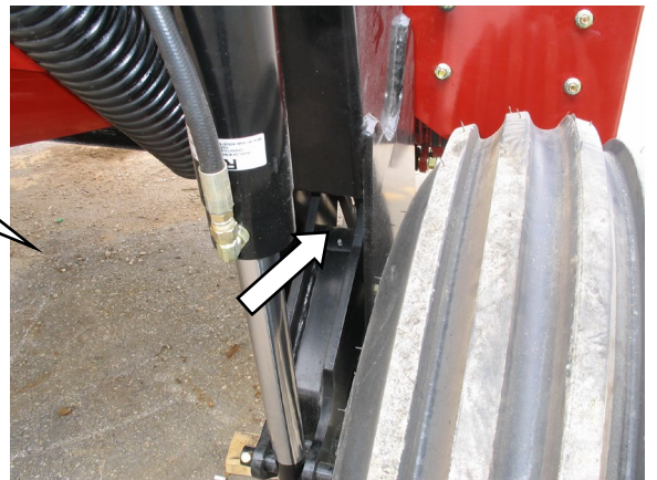
LIFT LINK 1PLC – BOTH SIDES
