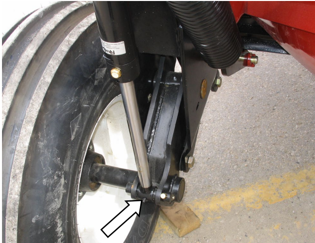
CYLINDER PIVOT 1 PLC – BOTH SIDES
