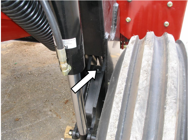
LIFT LINK 1PLC – BOTH SIDES
