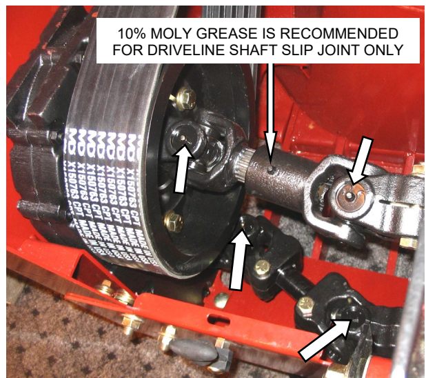
DRIVELINE UNIVERSALS (4 PLCS) DRIVELINE SHAFT (1 PLC)
