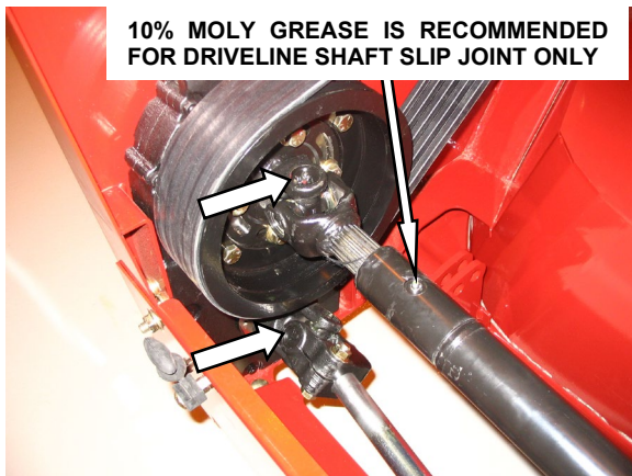
DRIVELINE UNIVERSALS (2 PLCS) DRIVELINE SHAFT (1 PLC)
