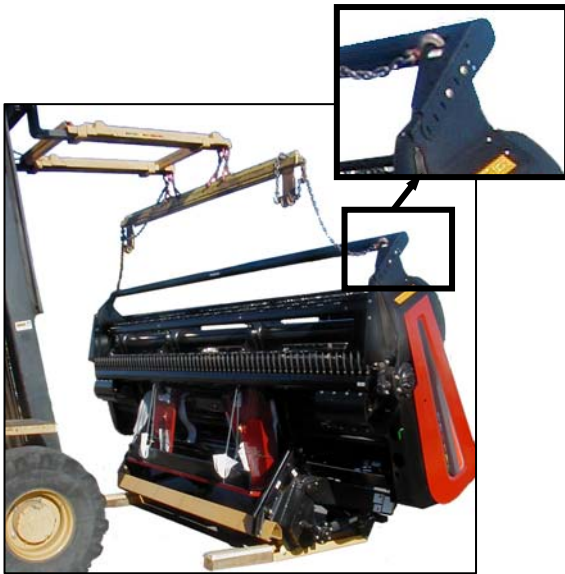
LOWERING HEADER WITH FORKLIFT
