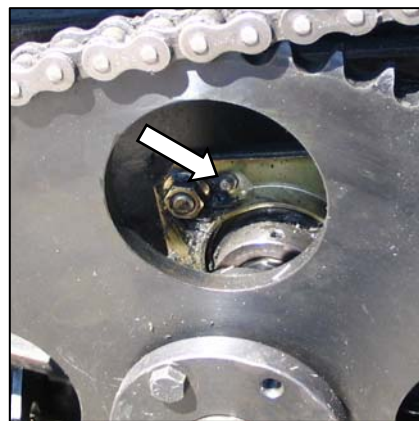
AUGER SHAFT BEARING - 1 PLC
