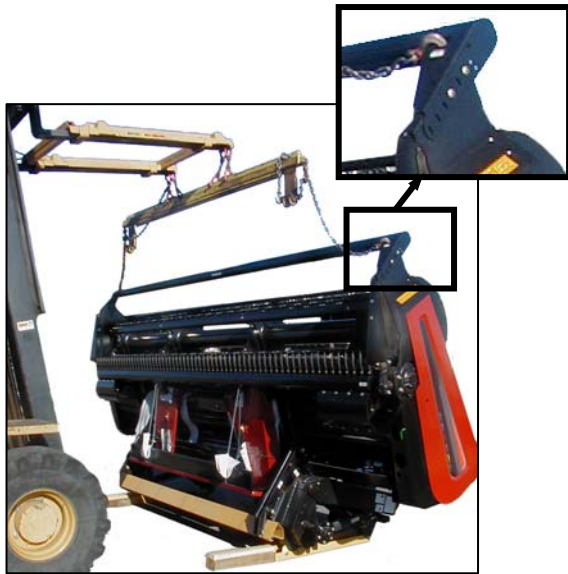
LOWERING HEADER WITH FORKLIFT
