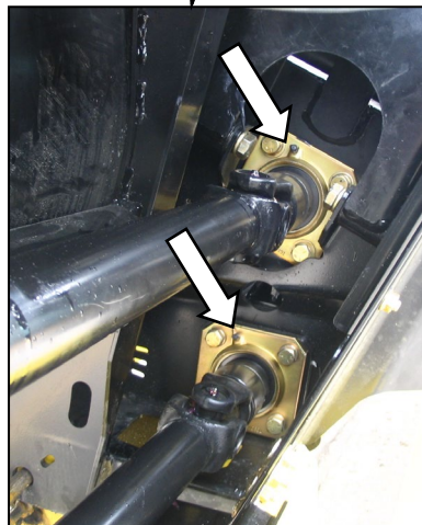
ROLL SHAFT BEARINGS - 2 PLCS
