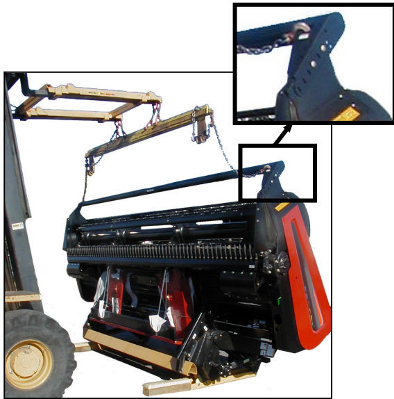
LOWERING HEADER WITH FORKLIFT
