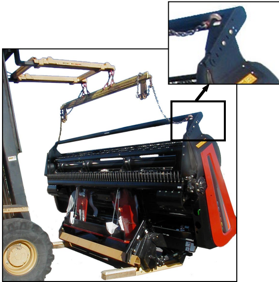
LOWERING HEADER WITH FORKLIFT
