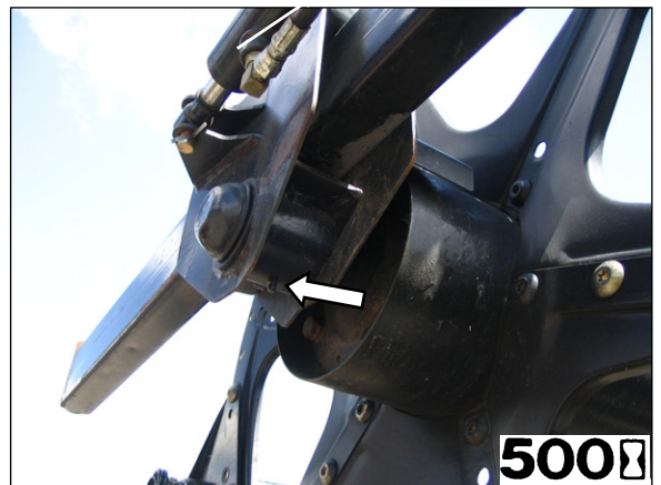
REEL SHAFT LH BEARING (1 PLC)
