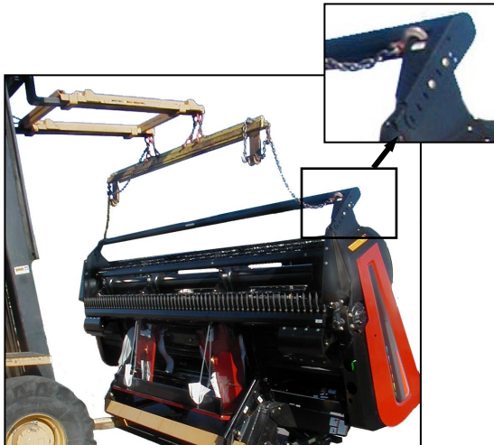
LOWERING HEADER WITH FORKLIFT
