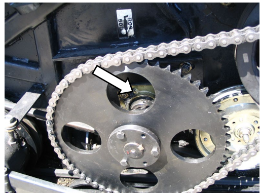
AUGER SHAFT BEARING (1 PLC)
