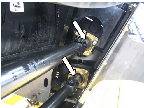
ROLL SHAFT BEARINGS (2 PLCS)
