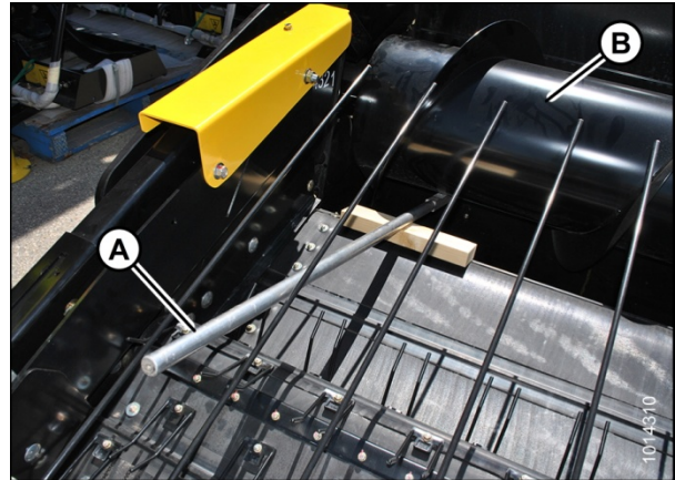
Figure 5: Pry Bar Supporting Auger
